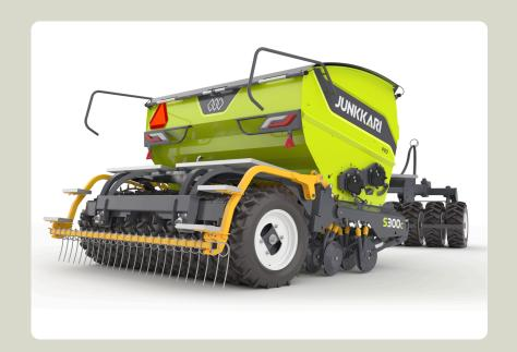
The coulter's long arm provides flexibility and ensures precise seed placement even as soil type varies.
