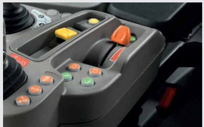
Electronic hand throttle with 2 engine memory speeds.
