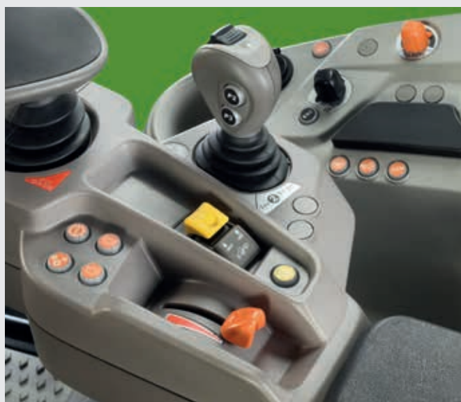
↑ Electronic joystick for front loader control.
