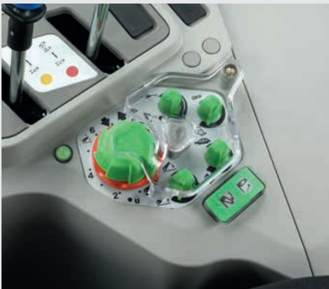
↑ Electronic rear lift controls.
