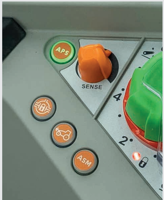
APS activation with adjustable response.
