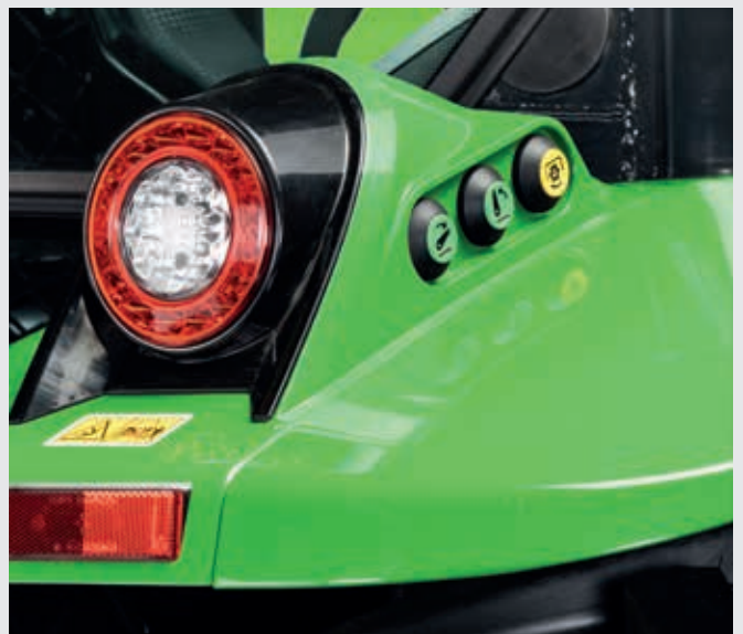
↑ External controls for PTO and rear lift.
