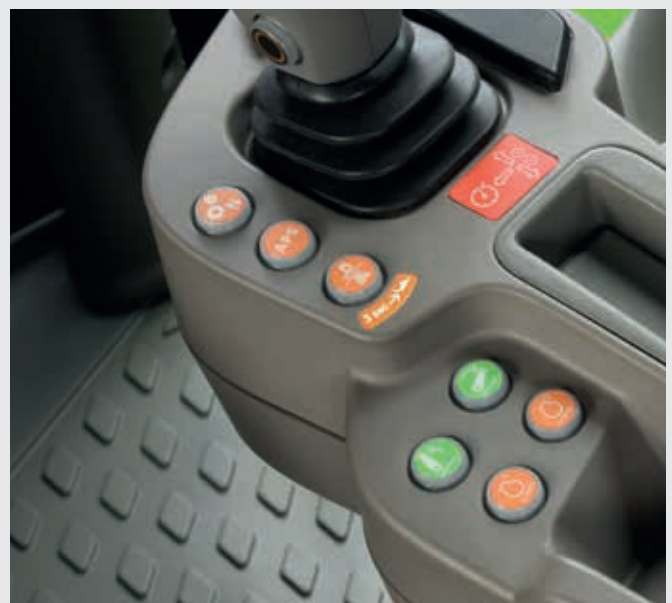
Transport, Field, Creep driving modes selection.
