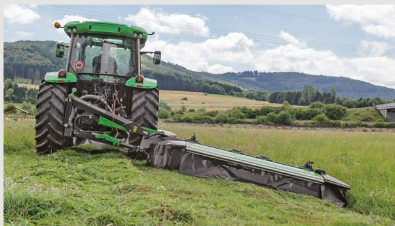
EXTREME POSSIBILITIES OF MOWING SLOPES, 30° UPWARDS AND 30° DOWNWARDS
