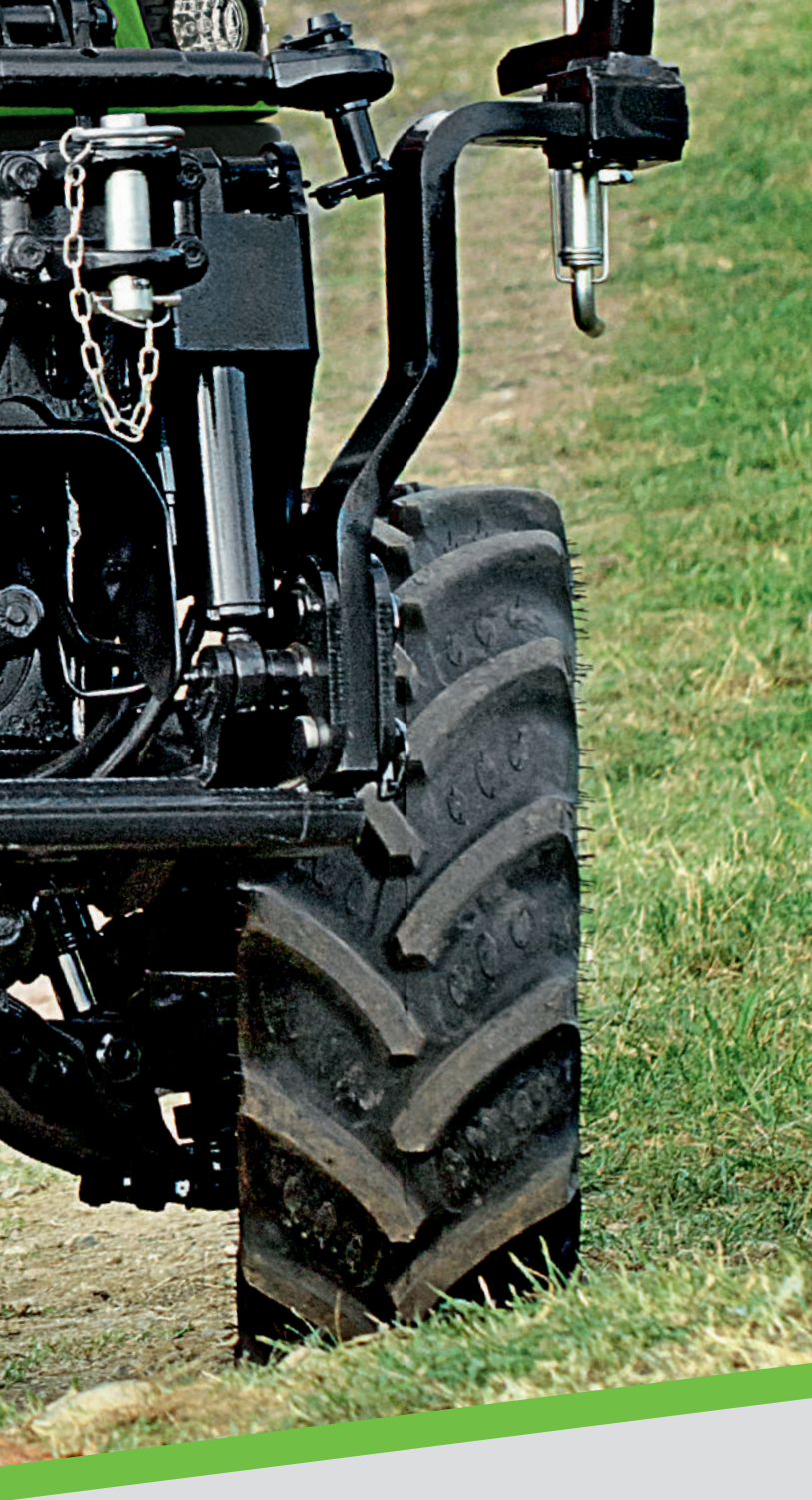
Improved turning radius thanks to a slimmer front support.
