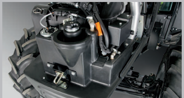
The fuel tank built into the front axle block can be filled with the bonnet closed, while an additional tank is located below the chassis.
