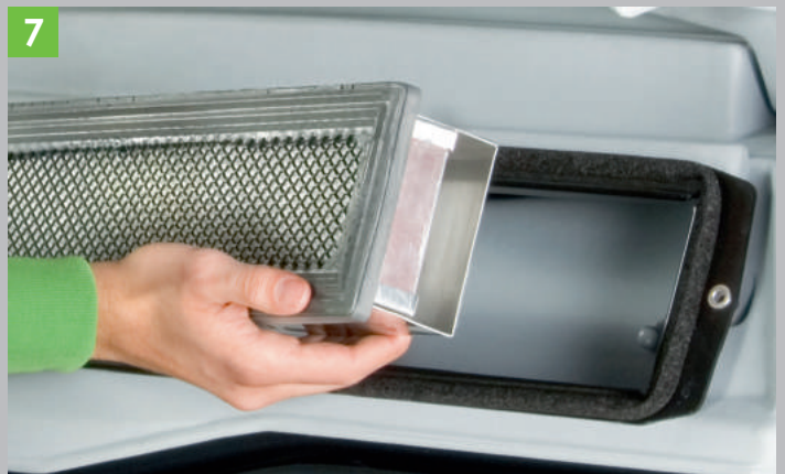
The cab air filter prevents dust and chemicals. Clean air inside the cab at all times.
