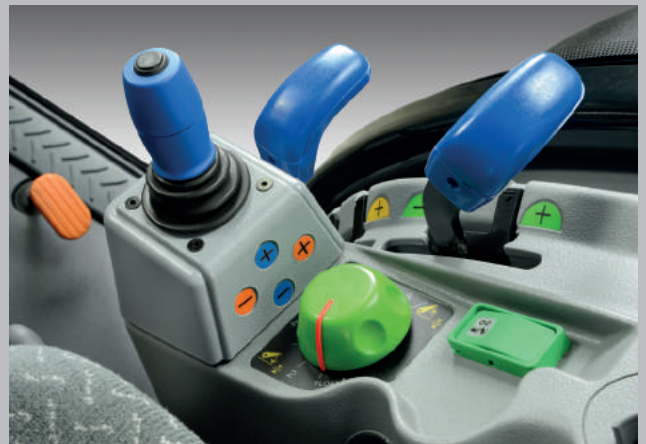
Controls for the rear power lift and hydraulic working equipment: close together and easy to access.
